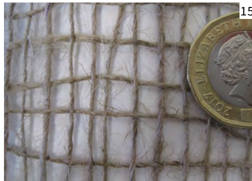
Figure 15: Modern hessian for producing traditional fibrous plaster, with a loose plain-woven fabric of twisted jute or hemp yarns. Plaster of Paris easily penetrates the widely spaced weave.
