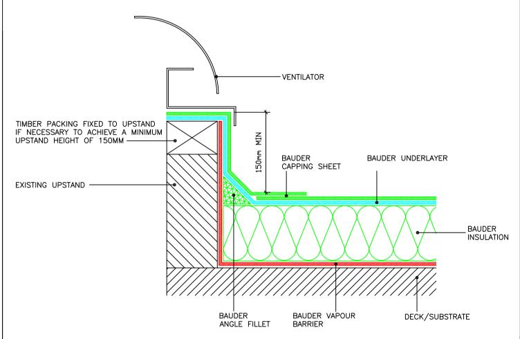
THIS IS A TYPICAL UPSTAND DETAIL WHICH CAN BE MODIFIED TO SUIT DIFFERENT STYLES OF VENTILATOR
