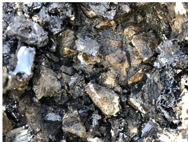
Chippings were found to wet between the layers of bitumen.
