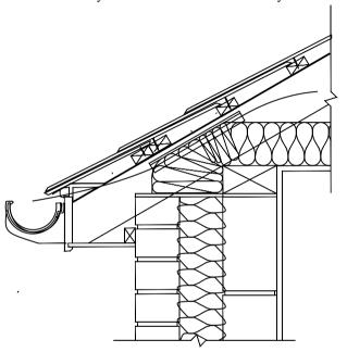
Fit grills and trays to ensure clear airflow over fascia and insulation and continuous support to form a drip into gutter.
