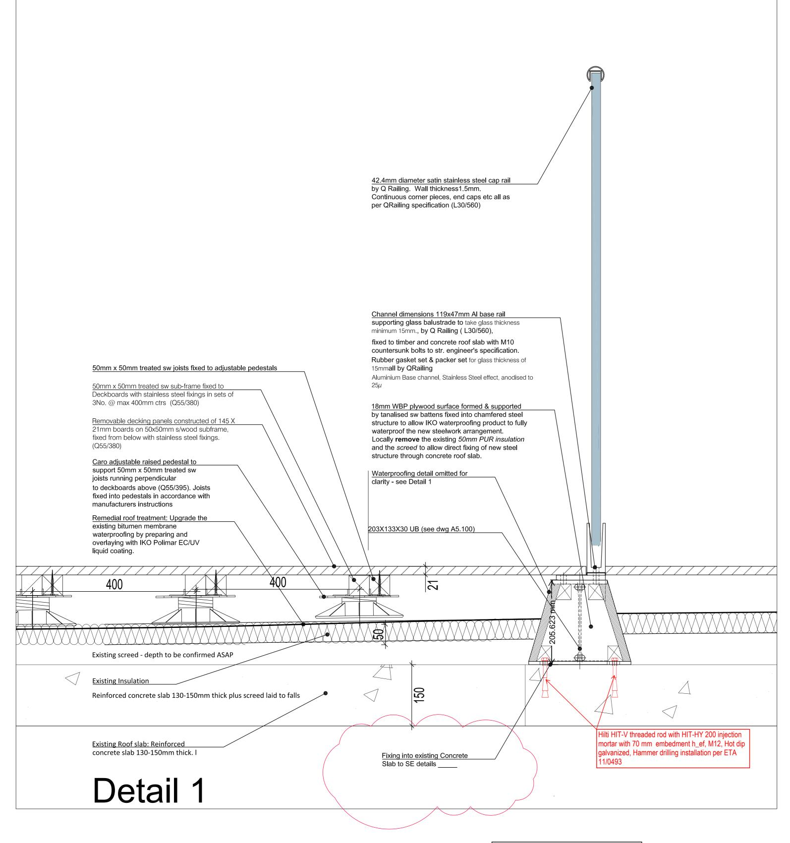
Easy glass Pro system with 21.52mm toughened laminated glass and a 48.3mm cap rail to the head of the glass - Proprietary balustrade system fixed to steelwork structure L<sup>30</sup>/<sub>560</sub> See Detail 1 Polimar UV Top Coat Polimar GRF Polimar EC Embedment Polimar KRM
