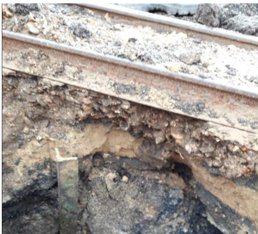
Photo 38: View of the track bed and made ground within TP14
