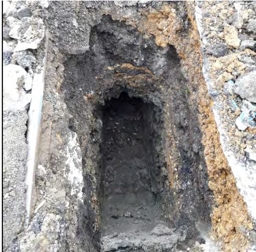
Photo 41: Groundwater seepage within TP15
