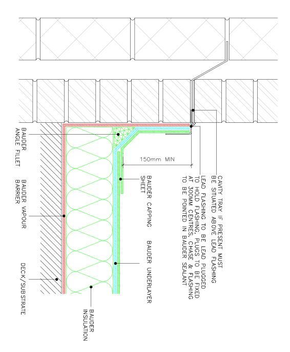
UPSTAND DETAIL TO BRICKWORK (UN-INSULATED CAVITY WALL)
