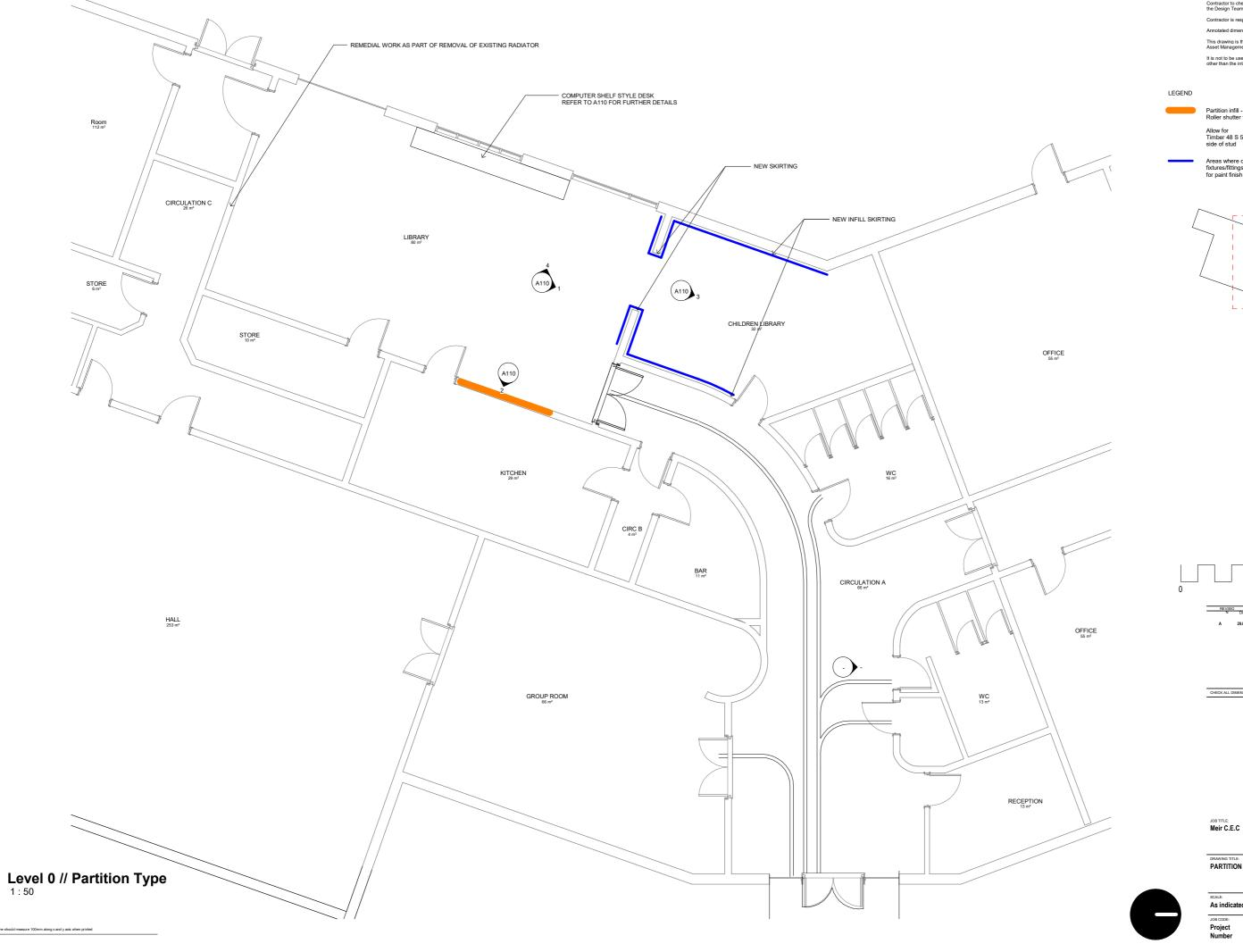
Partition infill - existing roller shutter opening to be infilled. Roller shutter to remain insitu with boarding to front face
