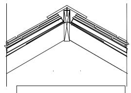
A length of underlay should be taken over the hip and overlap general underlay by 150 mm min.
