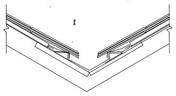
Provide suitable timber base 225 mm wide x 19 mm thick to either side of valley. The top of timber boards should be equal to either the top of the rafter or counterbatten if present
