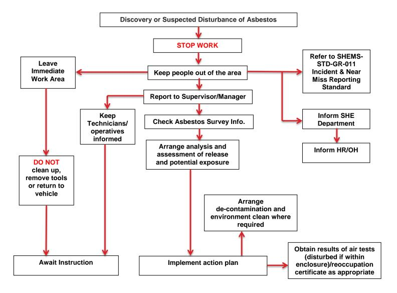
Accidental damage is any damage, in any form, to an ACM. Even minor disturbance may release fibres.
