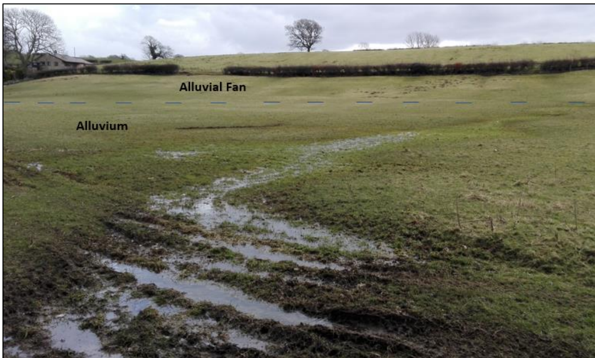
Figure 4-9 Evidence of high groundwater levels in alluvium along the River Conder (looking south). Approximate NGR 349196 456387.
