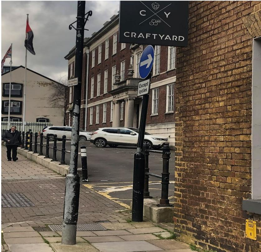
9. First of decorative lamp-posts – this is degraded with paint peeling off. On the floor by the lamp-post is a further Utilities access, with another at the exit point of the car access outside Old County Hall.
