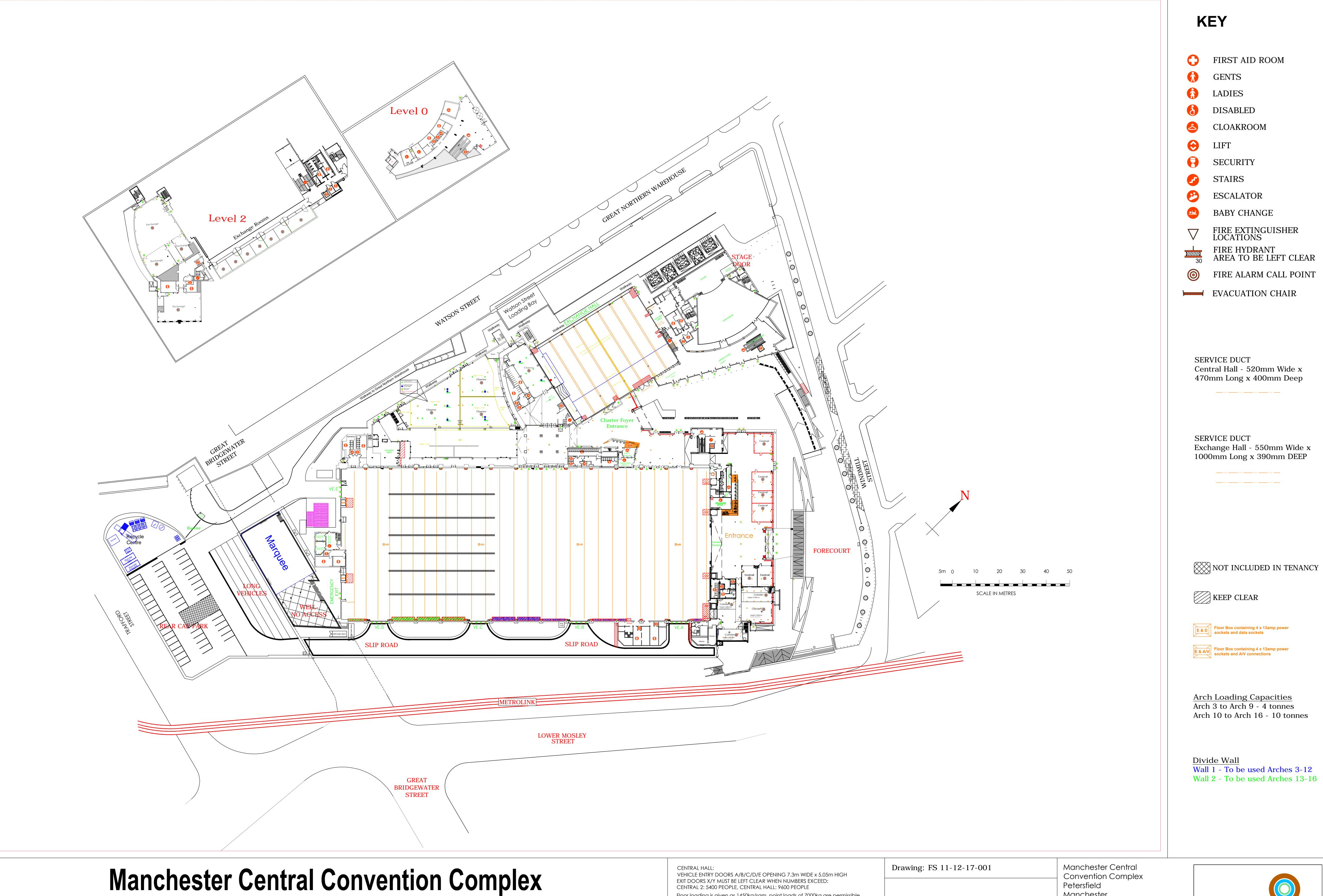
Floor loading is given as 1450kg/sqm, point loads of 7000kg are permissible 3m apart or at 2m distance from other distribution loads. Vehicles up to 4000kg gross weight are permitted in the hall. Loads & movements exceeding these limits must be verified in writing by the hall management:
