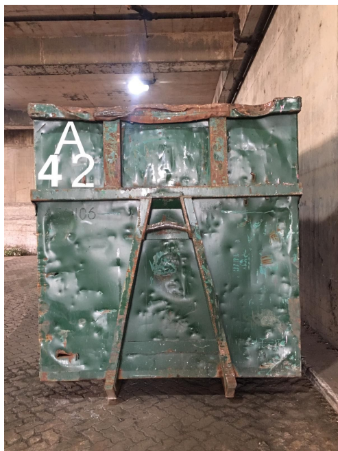
Photo 5 – bulk bins needing sections cut out and replaced and new tops rails
