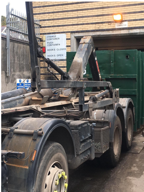
Photo 1 – hookloader vehicle - chassis & tipping system
