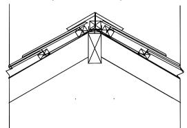
A length of underlay should be taken over the ridge and overlap general underlay by 150 mm min.
